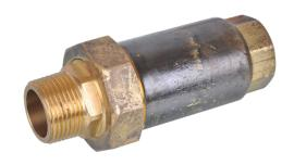
Dual Check Valves are utilised for protection from cross contamination of non potable water with potable water. They are used in low hazard conditions such as rain water tank systems and domestic meter connections.
