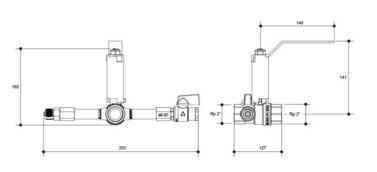
**Product Specifications** Watermarked Ball Valve HVAC with Extended Handle Extended Mini Ball Valve And Extended Test Point FI X FI **50MM**
