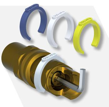
Provided with the "TRI-SET" selectable pressure limiting valve are three coloured plastic clips which indicate the valve's pressure setting. The pre set valve comes with a white clip fitted to indicate that the valve is set to 500 kPa. The yellow clip provided should be fitted if the valve is set to 350kPa and the blue clip fitted if the valve is set to 600kPa.
